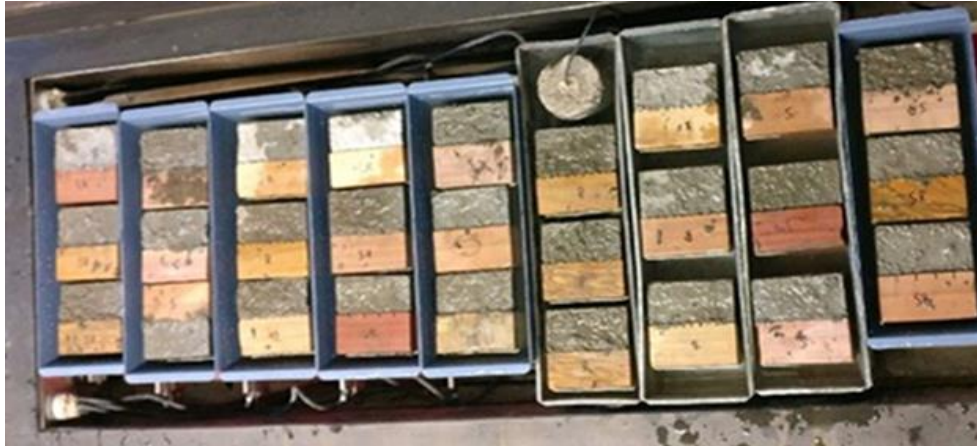
Figures 5: Specimens undergoing freeze - thaw cycles
