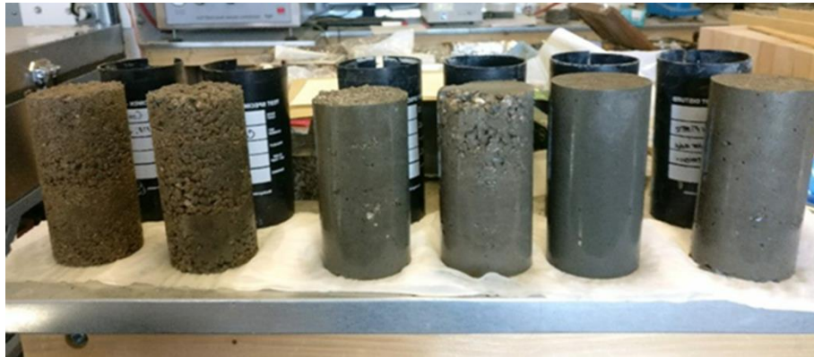
Figure 3: Specimens for preliminary testing, original design mix (farthest left), modification improvements (left to right)
