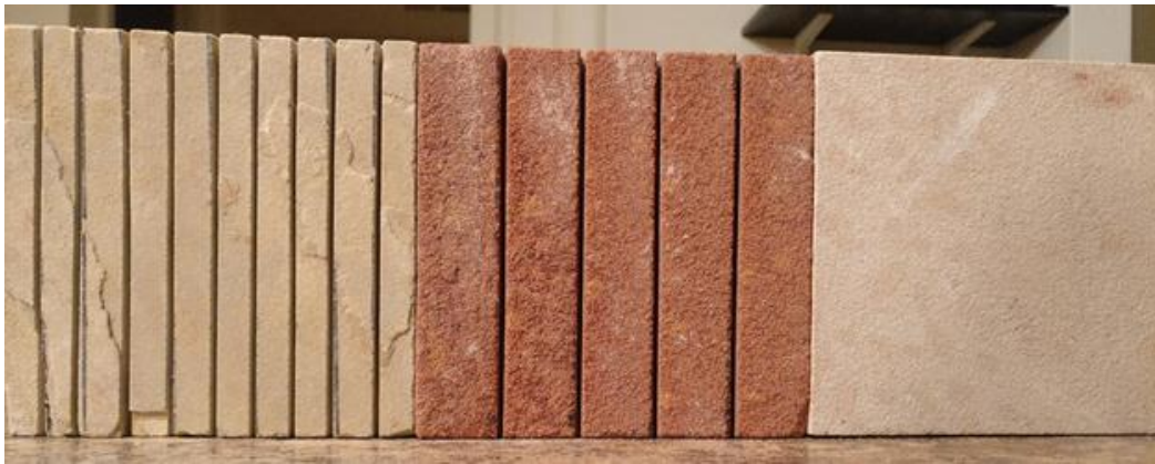
Figure 2: Flagstone surfaces: rough (left), semi-rough (middle), smooth (right)
