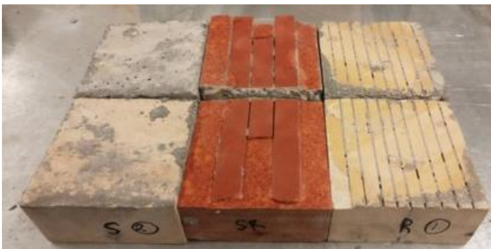
Figure 9: Representative control specimen failure planes of each type of surface roughness
