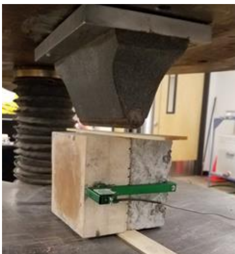
Figure 6: Specimen, before test, with placed extensometers on each side
